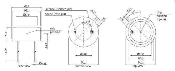
Selection Code "5" (photodiodes without filters) — TO5 Ni plated housing, 9.2 mm diameter, 4.3 mm height, two gold plated pins (Anode grounded and Cathode isolated).
