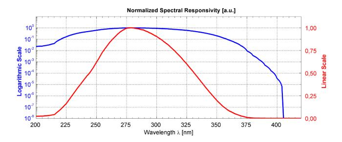
The curve's maximum is at approximately 280 nm. The response falls down to 10% of maximum at 221 nm, (UVC edge) and 358 nm, (UVA edge). Unfiltered SiC is the standard application and can be used for any UV measurements where the whole UV band needs to be measured or a quasi monochromatic UV source (such as low pressure lamps) is controlled.
