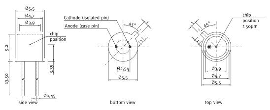
Selection code "18" — TO18 Ni plated housing, 5.5 mm diameter, 5.2 mm height two gold plated pins (Anode grounded and Cathode isolated).
