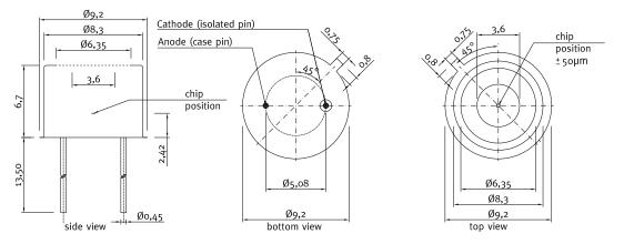
Selection Code "5" (photodiodes with filters) — TO5 Ni plated housing, 9.2 mm diameter, 6.7 mm height, two gold plated pins (Anode grounded and Cathode isolated).
