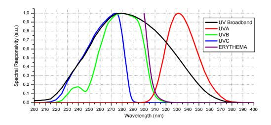
The graph assigns the filtered photodiode's spectral response to an individual wavelength. The following table extracts the most important specifications.
