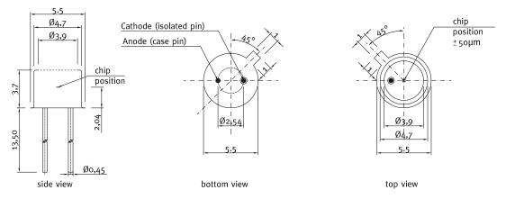
Selection code "18S" — TO18 Ni plated short housing, 5.5 mm diameter, 3.7 mm height two gold plated pins (Anode grounded and Cathode isolated). Not available with filters.
